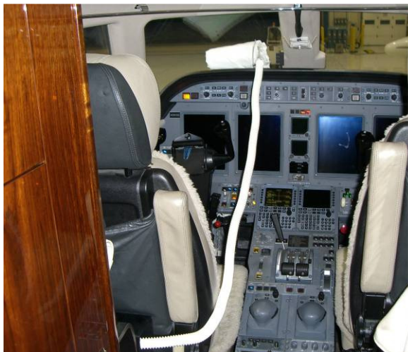
Wrapped IVU on Glare Shield for Left pilot Inboard deployment
