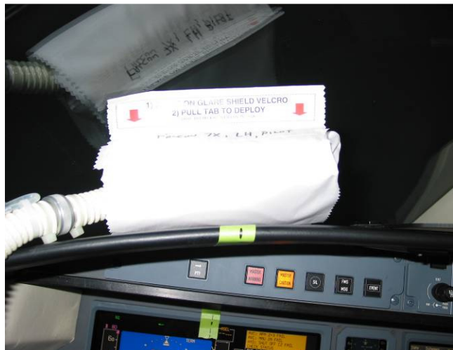
Wrapped IVU on Glare Shield For Left pilot Outboard deployment
