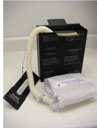
EVAS ® container with cover open & IVU out
