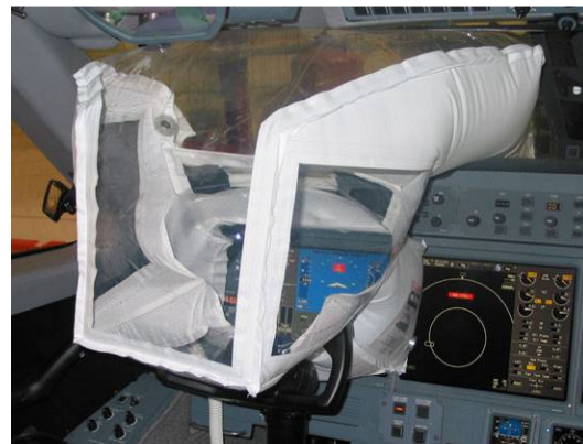
View of instruments through inflated IVU
