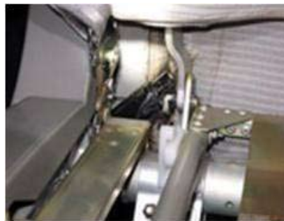
Photo shows burn marks found in a gap between the seat and the seat back on a Japan Airlines flight. At approximately 10,000 feet a flight attendant detected a burning smell in the back of the cabin.
