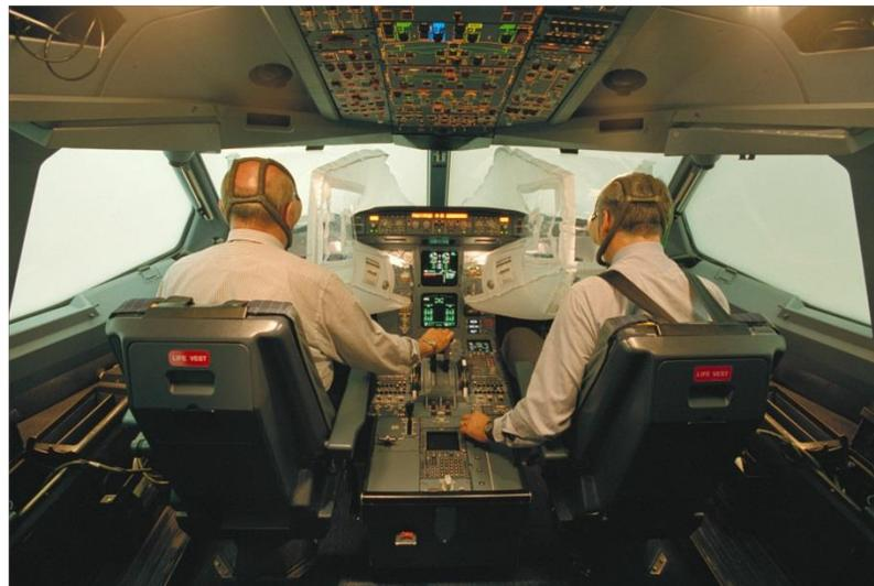
EVAS deployed in Airbus A330
